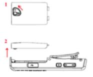
The serial number and IPUI number of each handset is situated either on a label behind the battery, or on the package label.
